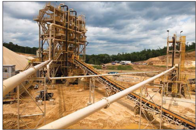
From bottom right, a conveyor carries sand from the crushing area to a wash plant tower to be washed and sorted by grain size at the Preferred Sands plant in Blair, Wis., on June 20, 2012. Lukas Keapproth/Wisconsin Center for Investigative Journalism
