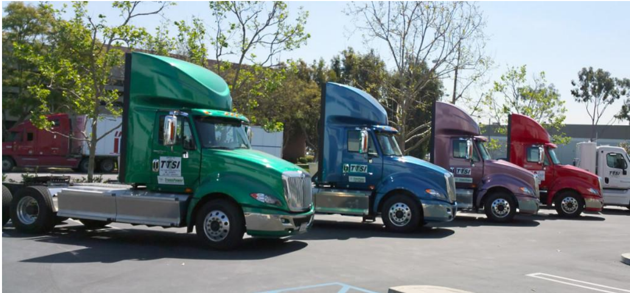
Figure V-4: Intercity electric Class 8 trucks with 80,000 pound capacity. Source: TransPower 2015, at http://www.transpowerusa.com/press-releases/16-million-in-new-orders-for-transpower-trucks-and-tractors .
