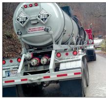
Tanker truck of hydrochloric acid to be used in the frack fluid.
