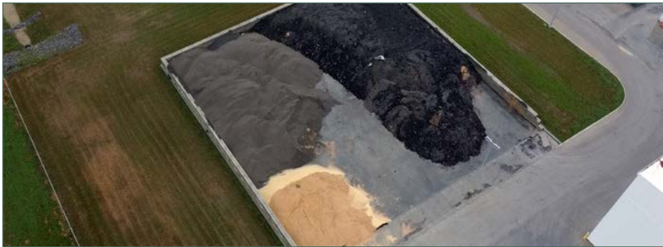
Photo taken in September above Rockwool's B170 Melt for Reuse area. Note the pile of light beige material. This is bauxite, a raw material naturally high in aluminum.
