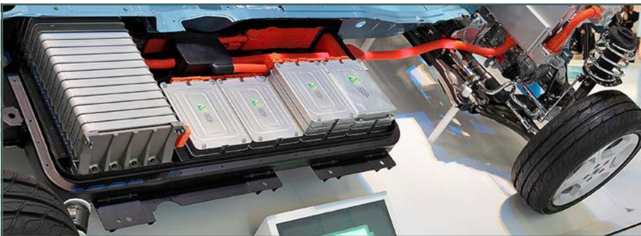
A cut-away view of the chassis of a Nissan Leaf EV showing the lithium ion battery.
