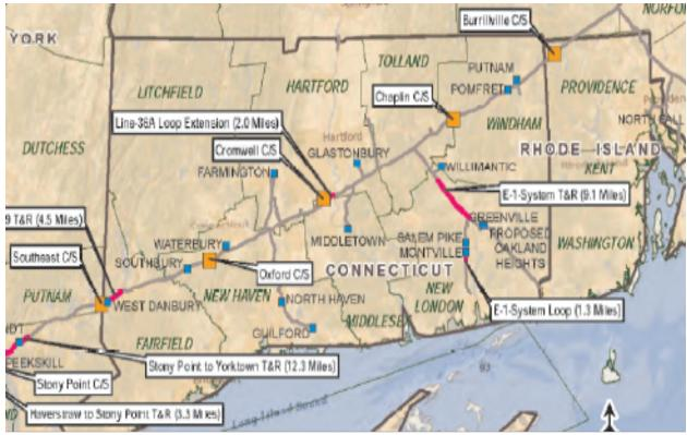
There are several compressor stations in Connecticut for this purpose. One compressor station is in Cromwell, one in Oxford, and one is located on the Mansfield –Chaplin line at 539 Tower Hill Rd. To measure gas flow, there are 13 metering and regulation stations in Connecticut. Every five to twelve miles along the pipeline, there are valves in case part of the pipeline has to be isolated.
