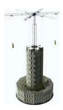
They convert excessive, unused electricity into potential energy which is a type of energy store with the potential to be turned back into electricity by driving a generator. Energy Vault's battery does this by stacking concrete blocks into an organized potential-energy-rich tower. The battery is charged by using that excess electricity to power crane motors which lift concrete blocks. The higher a block is lifted, the more potential energy it has stored.
