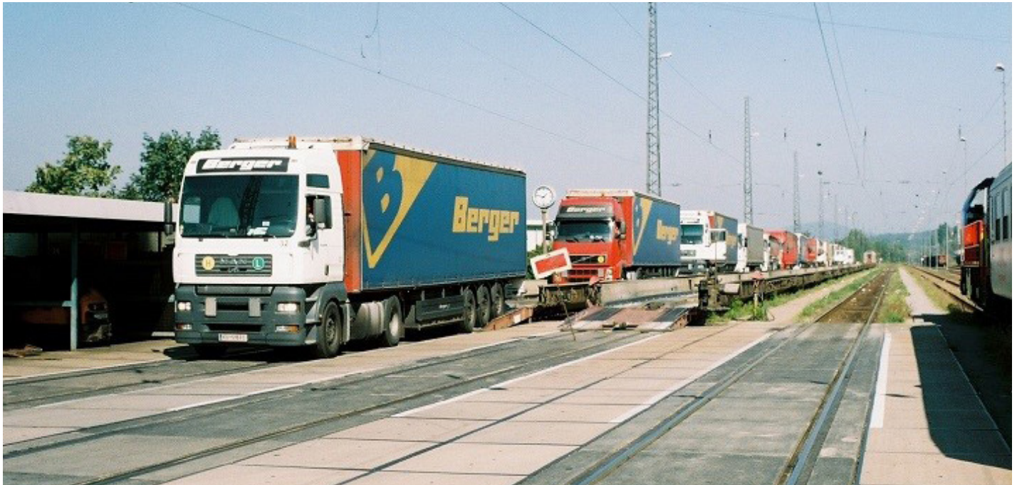
HUPAC INTERMODAL “ROLLING HIGHWAY” TRUCK-ON-TRAIN TERMINAL IN FRIEBURG, GERMANY (PHOTO: RAIL SOLUTION, DAVID FOSTER)
