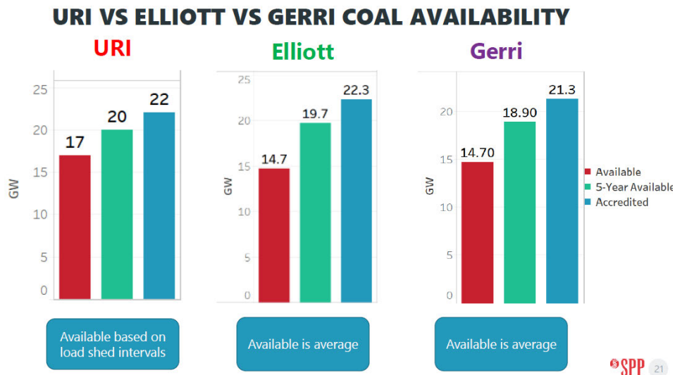
Figure 3: Coal Generator Availability During Recent Winter Storms 58
