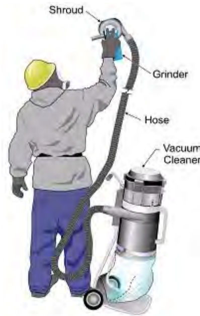
Grinder in use with the control in place
