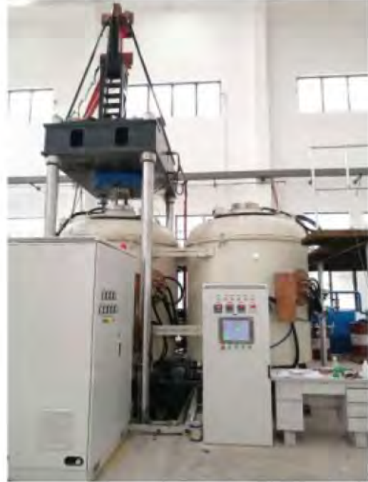
600T Vacuum Induction Hot Press Vacuum Heat Treat And Sintering Furnace 600T Vacuum Induction Hot Press Furnace for precise sintering. Advanced 600T...
