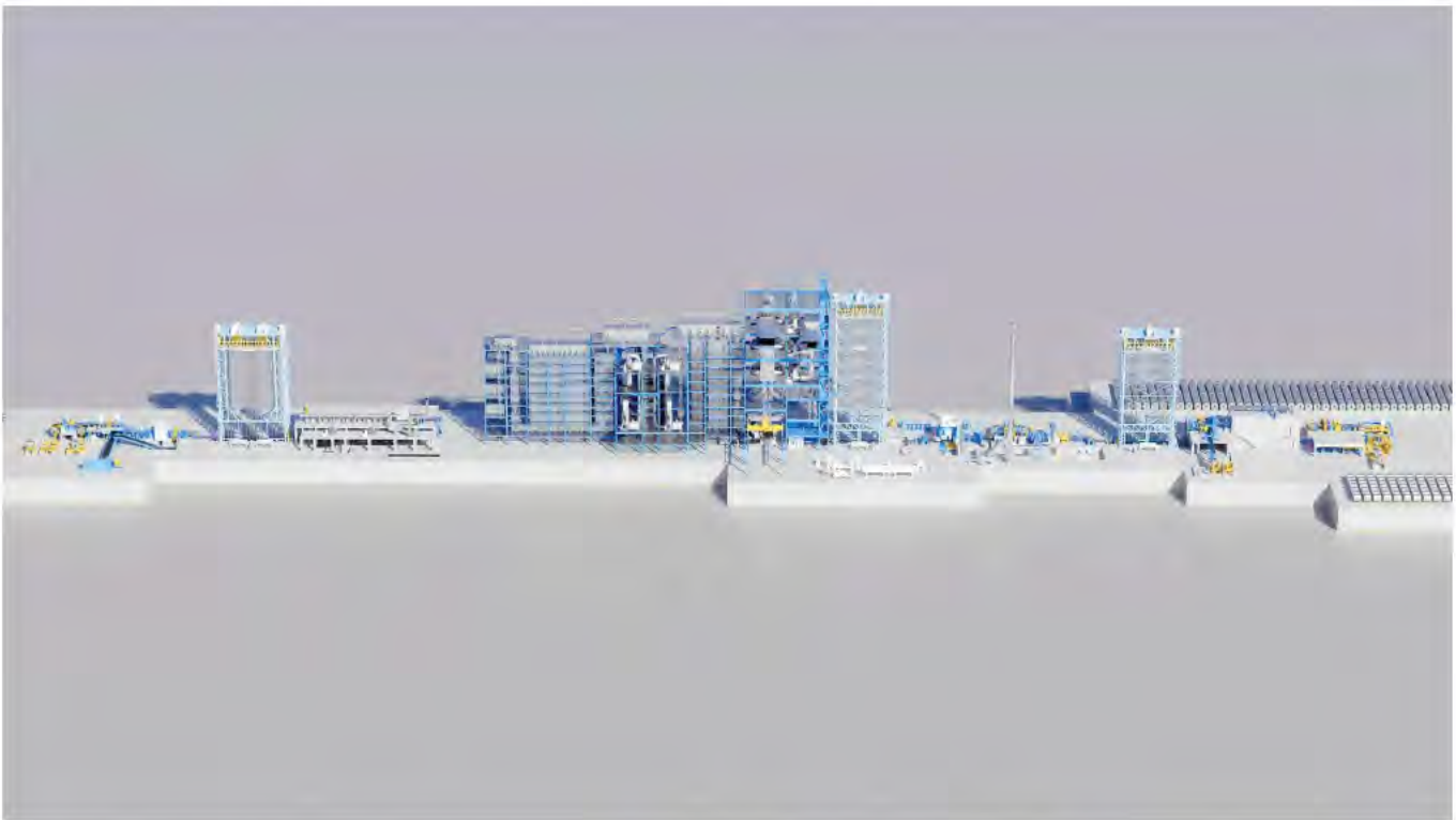
Rendering of the electrically heated continuous galvanizing line at SSAB, Sweden
