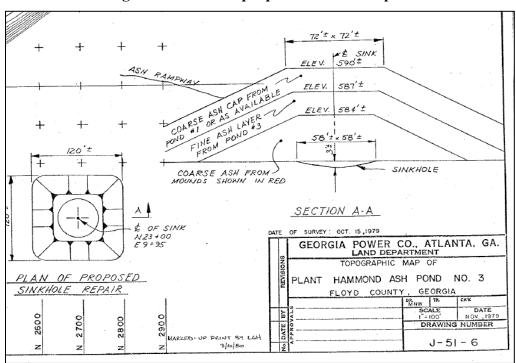
Figure 3. Details of proposed sinkhole repair
