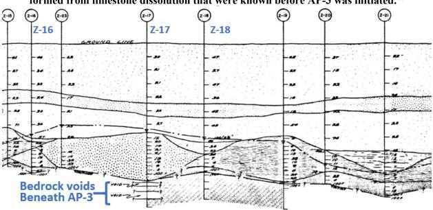
Figure 4. 1977 sketch of borings showing voids in the bedrock beneath AP-3 that have formed from limestone dissolution that were known before AP-3 was initiated.<sup>50</sup>
