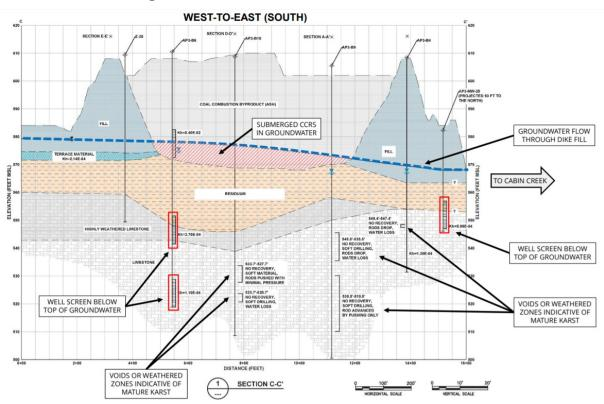
Figure 5. West to East Cross Section of AP-3.<sup>68</sup>
