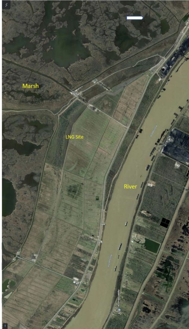
Figure 10. Google Earth image of the proposed LNG site on drained farm lands known as Deer Range Lake and at least -4.0 feet NAVD 88. Arrow points North.
