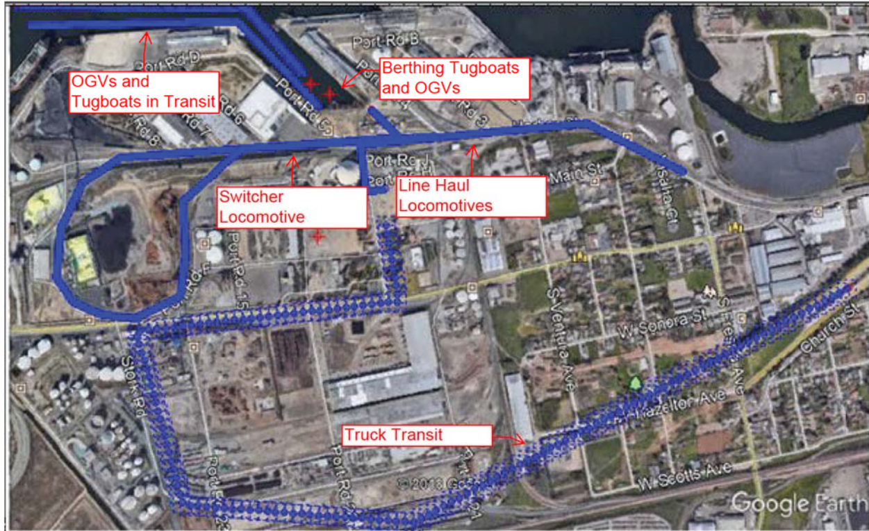
Figure 8: Case 1 – Location of Truck and Rail Routes Representing Shortest Distances Modeled in Revised HRA
