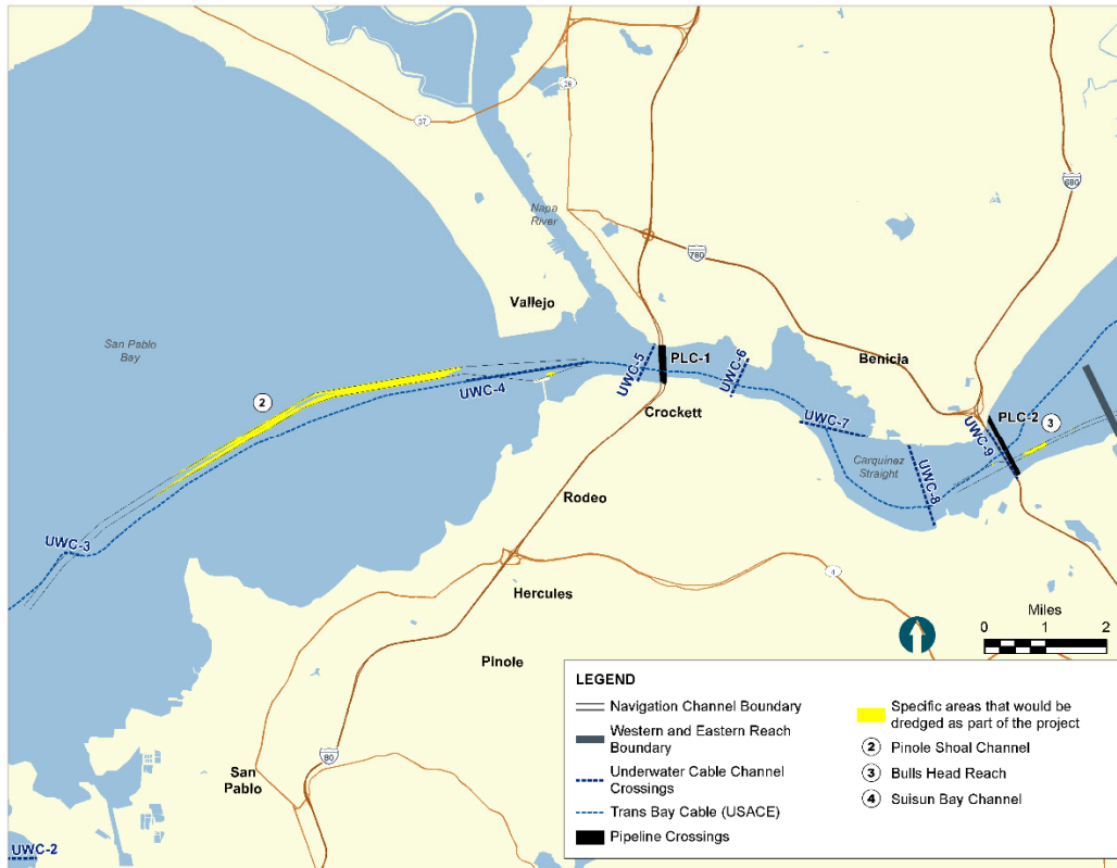
Figure 4-1. Dredged Area and Utility Crossings
