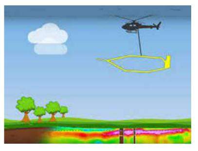
Survey data creates an image of the subsurface down to a depth of about 1,000 feet below ground surface and provides information about large-scale aquifer structures and geology. This information supports the implementation of local groundwater sustainability plans, which can help local agencies sustainably manage groundwater during drought.
