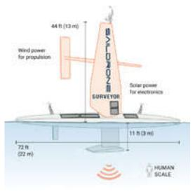
All these saildrones can be equipped with different measuring and recording devices. All are equipped with solar panels. A detailed view of Surveyor might get you ready to ask questions. It is offered with these options: positioning, deep-water bathymetry, shallow water bathymetry, wind speed & direction, barometric pressure, ocean currents, fish biomass, sound velocity profiler, and a surface
