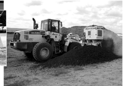
The compost turner attaches to the front of a Komatsu WA320-5 wheel loader. E 3 BioFuels also uses the WA320 as a general machine to help out around the ethanol plant.
