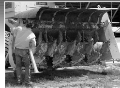
E 3 BioFuels mounts this turning attachment on its Komatsu WA320-5 wheel loader to create compost.
