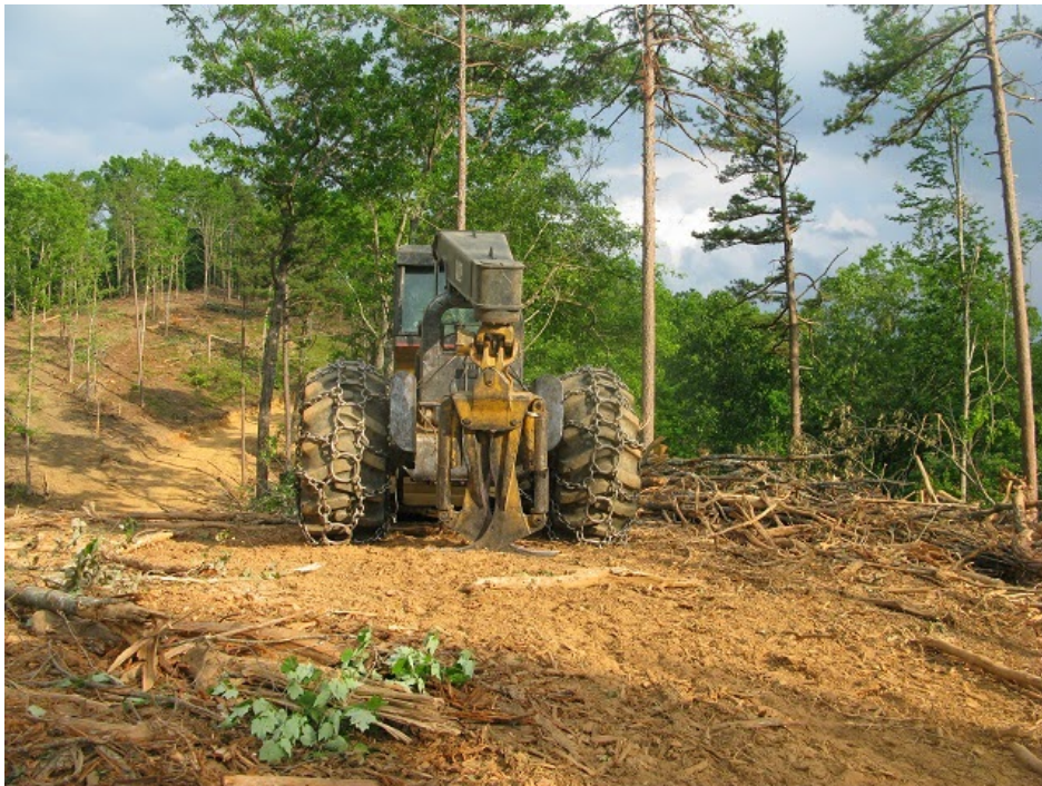
The Skidder that drags the logs to a central loading point. Note the huge chains on the wheels. They provide traction but have heavy impacts on the land.
