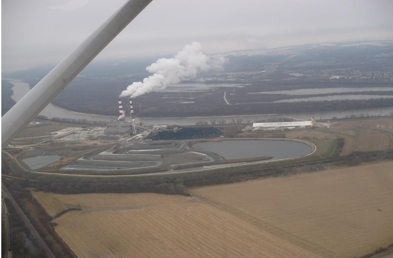
Edwards Coal Fired Power Plant on the Illinois River south of Bartonville off Route 24 and across the river from Pekin: coal ash ponds above.
