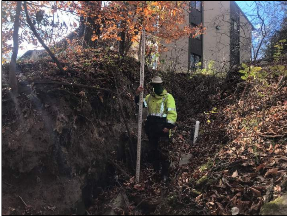
Photo 15: Reach 10, looking at side channel near the corner of Tamar Drive and Route 175, 7' eroding bank where apartment complex outfall meets Reach 10.
