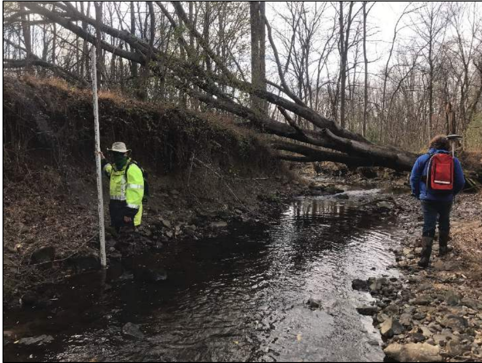
Photo 21: Reach 15A, looking downstream near confluence with Reach 16, 8' actively eroding bank and large fallen tree.
