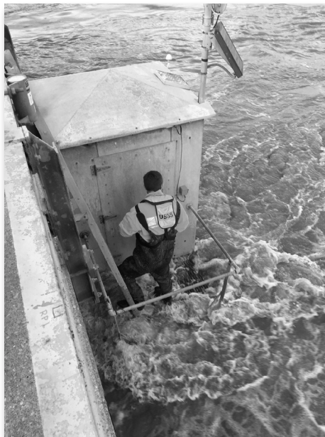
Missouri stream gauge is checked by staff. River forecasting is vital to the protection of life and property. Photo courtesy of the US Geological Survey
