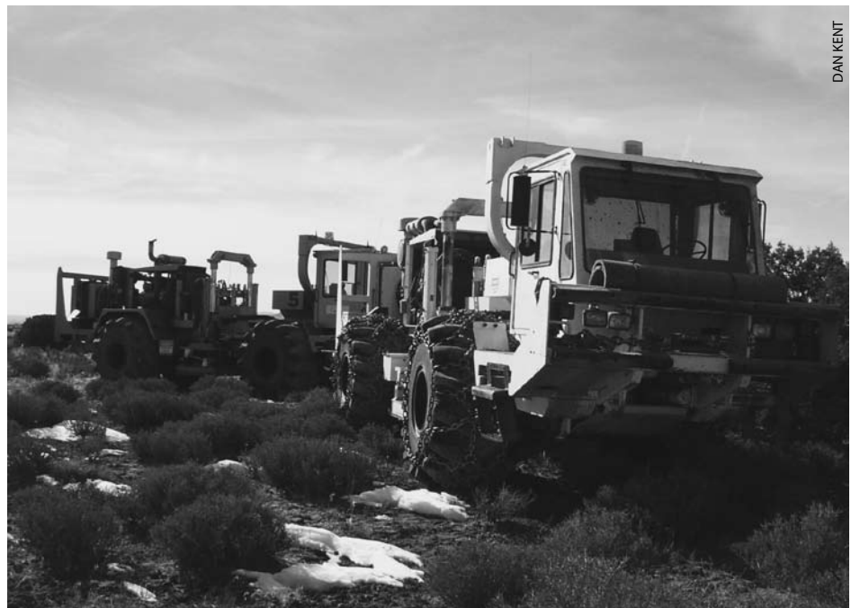
Huge seismic buggies on the Dome Plateau. These vehicles travel cross country to create vibrations to find oil and gas. You will note one has large chains on the tires. This was not allowed in seismic exploration permit.
