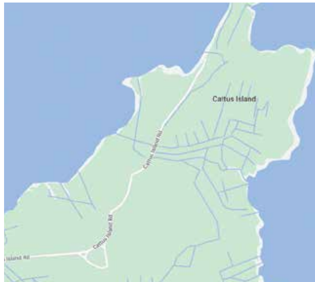
Cattus Island in Toms River has many trenches dug into it to drain standing water and prevent mosquito infestations. Credit: Google Maps Image: ©2022 Google.
