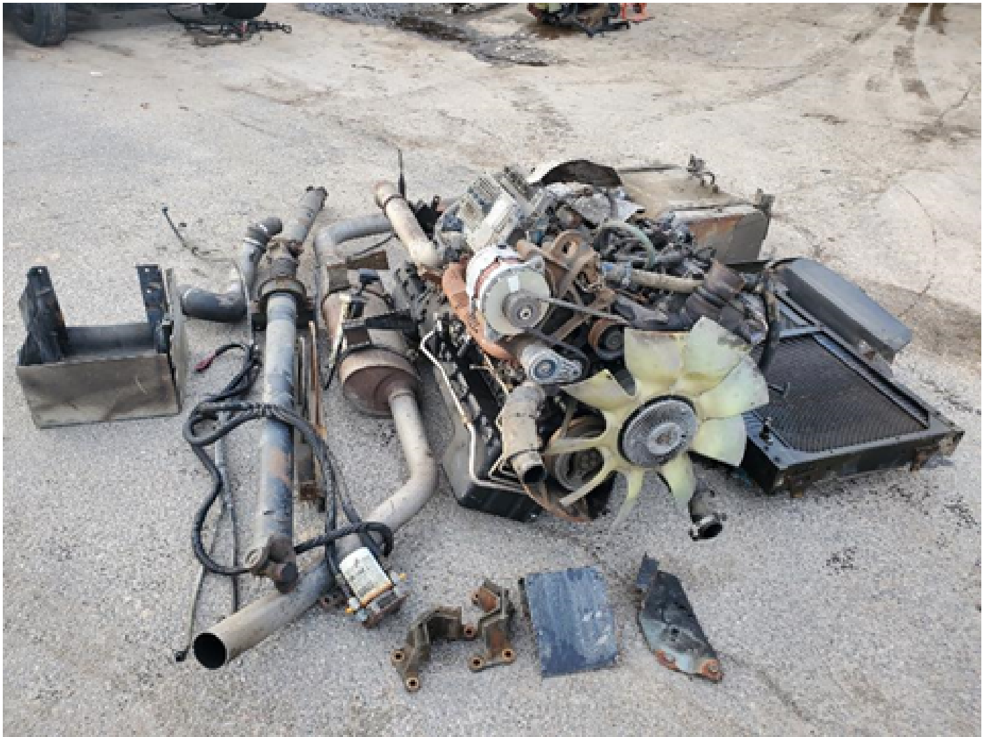
Diesel engine and drivetrain parts are removed from a repowered electric bus. Photo by Unique Electric Solutions.
