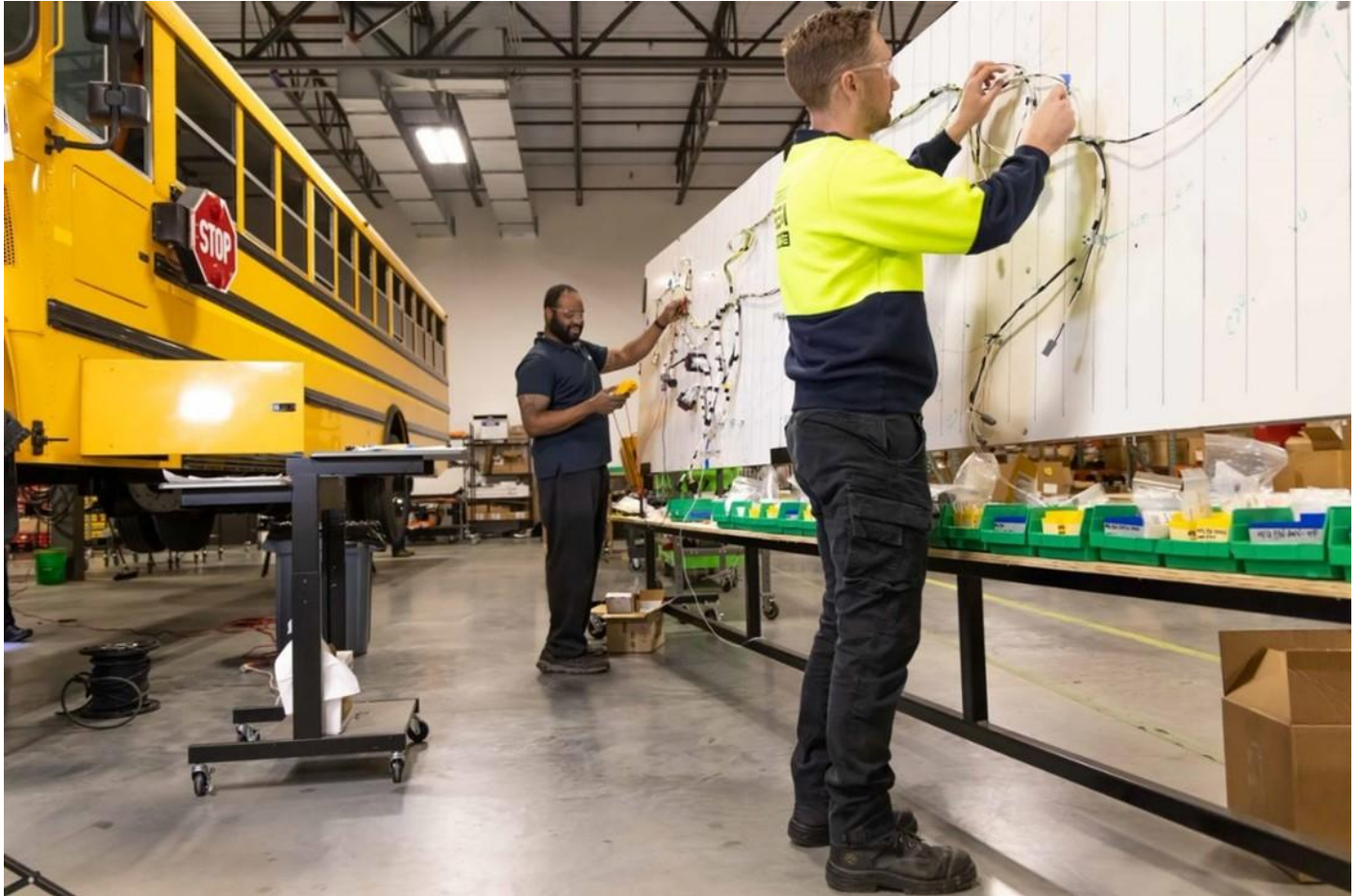
Technicians assemble a wiring harness for a school bus repower. Photo by SEA Electric.
